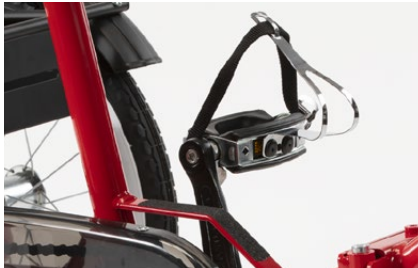
840 Pedal cage with strap. To keep the forefoot positioned on the pedal.
