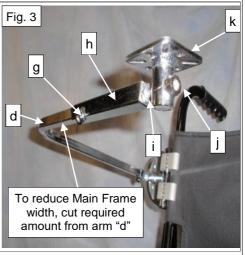
Frame using a hacksaw, finally clearing any swarf before re-installing into Rotation Mount. \* **NOTE:** The installer may wish to attach the Chin / Remote Controller to the Swivel Mounting Plate **(k)** Fig.3, at this stage whilst removed from the Main Frame.
