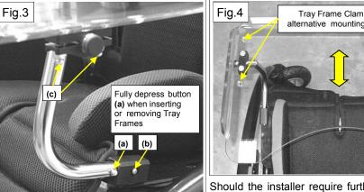
Tray Frame Clamps with alternative mounting positions
