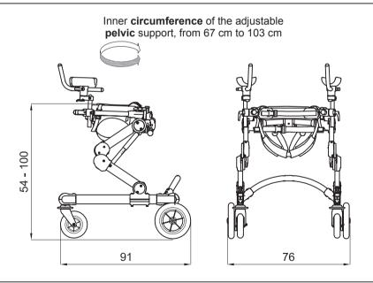
GRILLO POSTERIOR gait trainer size ThreeFour WEIGHT 17,7kg MAX LOAD. kg 90
